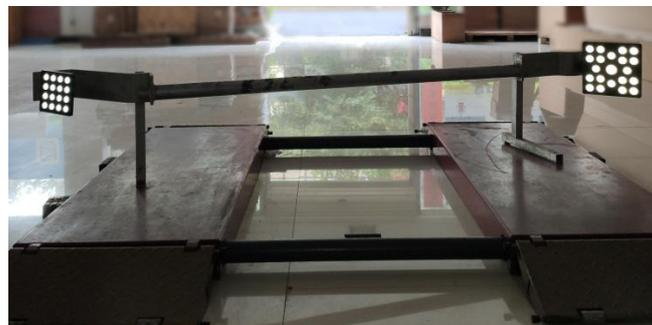
Let both targets be as closer to the center of views as possible. Adjust the position until the message says both targets' position is OK. Click "next" button to move to step 8.
