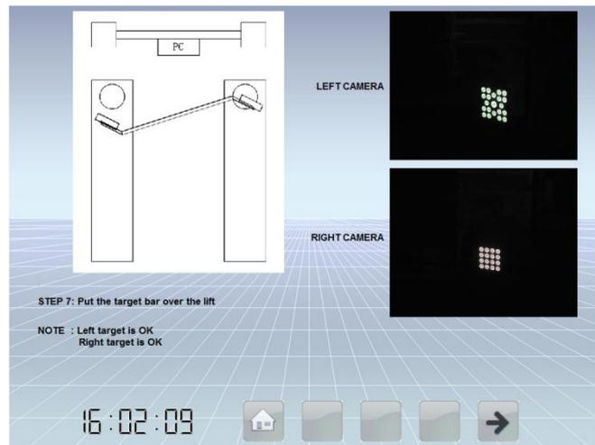
Move the stick back until the message says both targets' position is OK. Click "next" button to move to step 9. Again move the stick back until the message says both targets' position is OK. Click "next" button to complete the RCP calibration.
